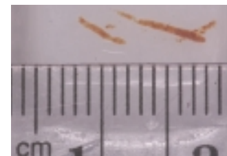
Photo 3. Borderline specimen. While this specimen has the necessary length, there may be an inadequate volume, depending upon the amount of material that has been "sliced" off the block to make slides. The laboratory would attempt to perform metals analysis on this specimen.
